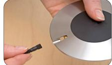
The MicroDot connector is assembled from the topside of the microphone.
